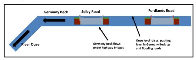
A smaller stream, Tunnel Drain, is piped below the Fordlands Road community and drains into Germany Beck by the Selby Road bridge. Significant rainfall and raised River Ouse and Germany Beck levels can increase the flood risk to a number of properties in the community. Emergency response procedures have been carried out to minimise this risk in a number of flood events, most recently in February 2020.
