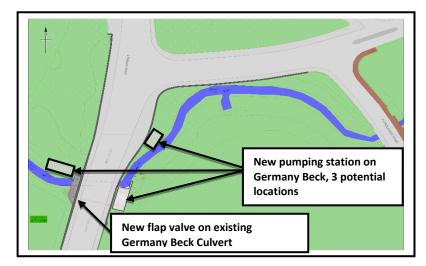
CYC have worked with consultants working across the city wide programme of interventions and have a high level design for a pumping station that would allow Germany Beck to drain effectively even when flood levels are high on the River Ouse. Pumping would maintain low levels in the beck and Tunnel Drain as
